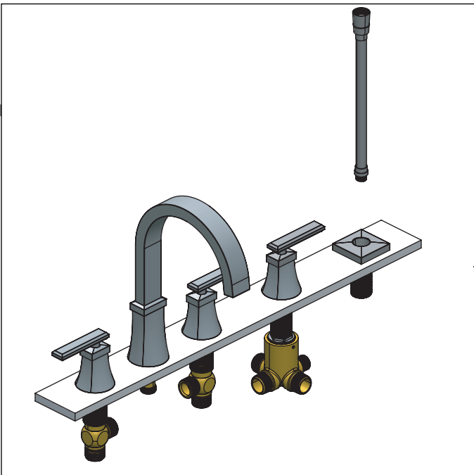
Drop hose down through deck hole
