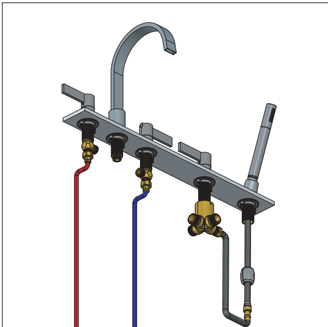
Connect hot & cold-side connection
